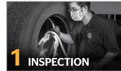
1 INSPECTION Thorough initial casing inspection, using state-of-the-art technology.
