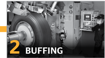
2 BUFFING Precise buff contours and consistent under tread thickness by computer controlled buffing.
