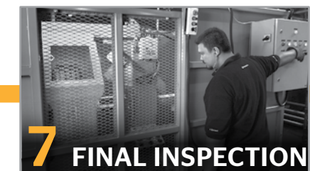
7 FINAL INSPECTION Detailed final inspection, ending with high pressure testing.
