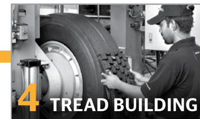
4 TREAD BUILDING Optimum casing fitting, ensured by laser guided tread application.
