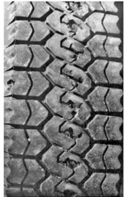
Example of Dyno Damage
